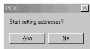
In setting addresses every addresses of ballast are deleted (information about groups stay save) and is done new assigning af addresses for the ballasts. If every founded ballast has its short address there is shown form for assigning ballasts into channels (groups).
